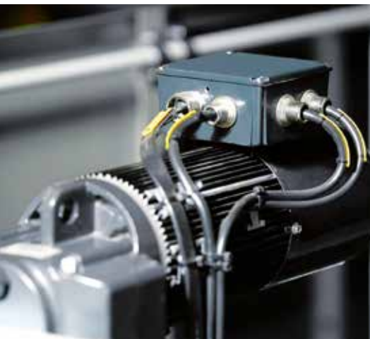
Trolley travelling motor with PIOTEX type wire marking
